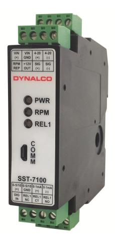
The SST-7000 series accepts a pulsed input and provides an extremely accurate 4 – 20 mA output representing speed of rotating machinery for a local panel meter or PLC analog input card. The SST-7100 also provides a quick relay response to over / under speed conditions. Applications include speed measurement & overspeed protection of industrial engines, turbomachinery and pumps.
